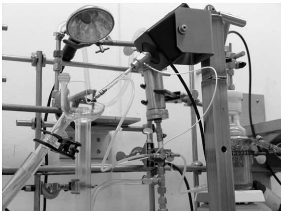
Fig. 1. Modified internal gelation system for use with SiC.
